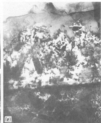
Figure 6 Microstructures from bulk composite material, after heat treatment for (a) 2 h at 600 °C, dislocation sub-grains and \alpha\text{FeSiAl} intermetallics in the aluminium alloy matrix, (b) 2 h at 700 °C, showing precipitated \text{Al}_4\text{C}_3 at a fibre/matrix interface, (c–e) 2 h at 700 °C, showing varying degrees of interaction at the fibre/matrix interfaces.
